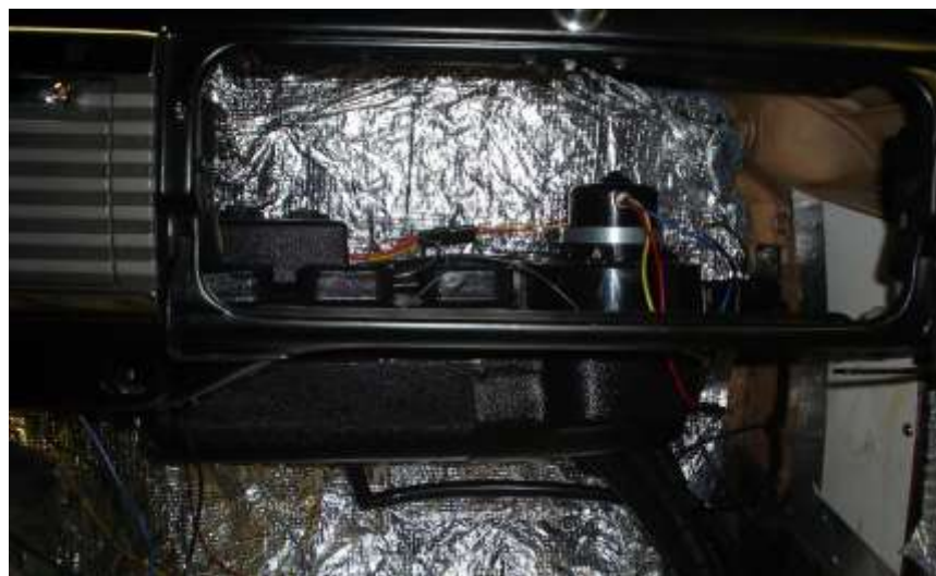
5/16 Bolt through the hood hinge for the evaporator bracket
