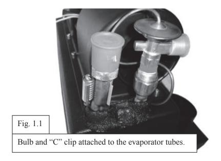
6) After the expansion valve bulb and "C" clip are attached place some black insulation (cork) tape over the tubes and expansion valve. Do not cover the threads or hex area of the tube. More tape will be needed later to cover all the connections and fittings.
