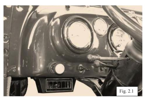
3) The vent and stock defrost outlets require duct hose to be attached to them. The hose will push over the ends of outlets. The dash vent has an oval outlet, the duct hose can be pushed down to fit over the oval. We recommend using screws or "zip ties" to secure
