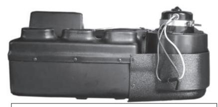
This is how the ID260 / 265 will sit in the vehicle. The right side has a hose cover below the blower motor housing. This is the view of the unit if you were sitting in the passenger seat.
