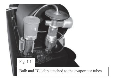
9) After the expansion valve bulb and "C" clip are attached place some black insulation (cork) tape over the tubes and expansion valve. Do not cover the threads or hex area of the tube. More tape will be needed later to cover all the connections and fittings.
