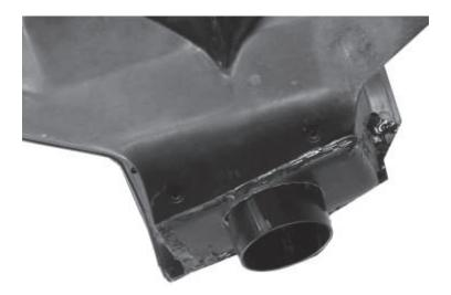
The above pictures illustrate the original defrost duct with a vent hose adapter. The picture is for illustration purposes only. The adapter for the Ford truck is designed to slide into the rectangle.
