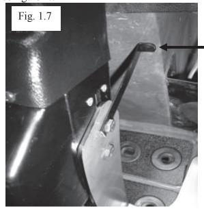
Support bracket screw into glove box.
