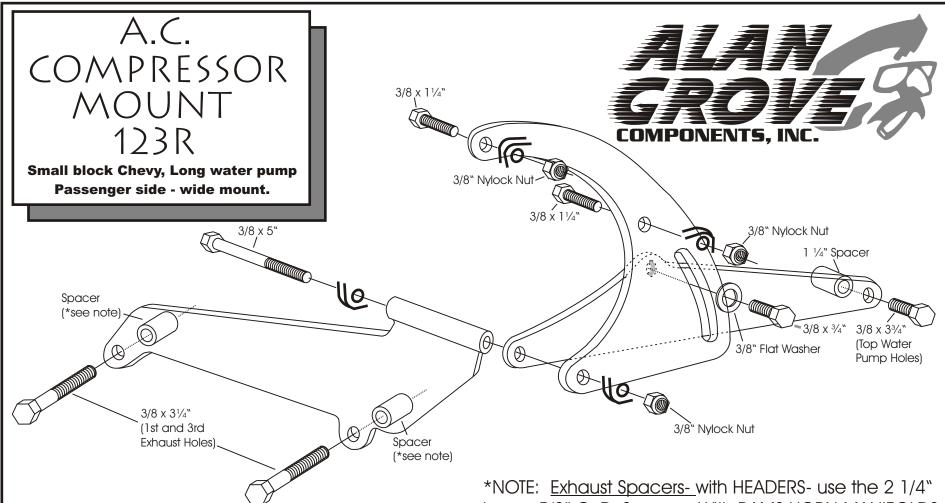
The compressor belt will run in the outer grooves of the crank and water pump pulleys originally used for the factory alternator. It was designed to be used with our 223L Driver's Side Alternator Mount.
