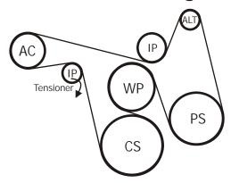
\*BELT DISCLAIMER: The belt included in this bracket kit is designed for standard 105 amp. Alternator applications. If your application is using the optional high output 130-145 amp. alternator; a smaller idler pulley at the factory alternator mount will be necessary for proper fitment of the included 6 rib belt (SEE ALTERNATOR DIMENSIONS ON FRONT PAGE). This smaller idler pulley is readily available at any auto parts store listed under part numbers:
