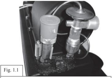
Bulb and "C" clip attached to the evaporator tubes.
