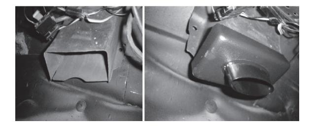
The above pictures illustrate the original defrost duct with a vent hose adapter. If you vehicle has two separate defrost diffusers the setup will be different than the one pictures. If the evaporator has four outlets the defrost Y with flap will be necessary to duct the defrosters.
