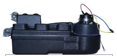
This is how the ID260V / 270 will sit in the vehicle. The right side has a hose cover below the blower motor housing. This is the view of the unit if you were sitting in the passenger seat.
