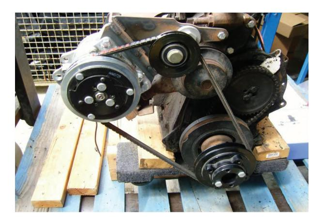
After the engine bracket, belts, and idler are installed the engine should look like the picture.
