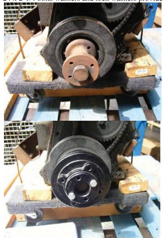
8) Reinstall the fan on the new crank pulley with the original hardware.
