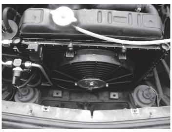
4) The electric fan should be wired up through a relay, below is a diagram for wiring up the Relay. When wiring the fan up; make the sure the fan is pushing air. The fan is reversible so the ground can be the hot and the hot can be the ground.
