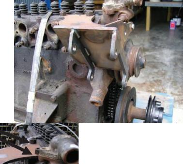
Use the two existing head bolts to secure the top of the bracket.
