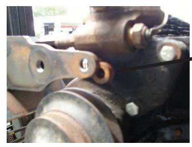
Use the 1/8" water pump spacer between the bracket and the water pump
